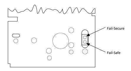
The modified Schlage mortise lockset is field reversible. Moving the pin from one position to another will change the function from fail-safe to fail-secure as illustrated.
